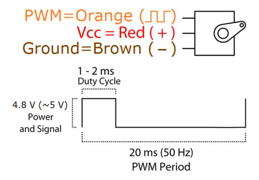
Position "0" (1.5 ms pulse) is middle, "90" ( $\sim$ 2 ms pulse) is all the way to the right, "-90" ( $\sim$ 1 ms pulse) is all the way to the left.
